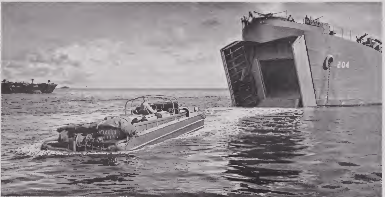
FIGURE 9. DUKW loaded with 105-mm shells, leaving LST off Noemfoor Island. Offshore reefs obliged landing ships to remain afloat while they were discharged by DUKWs which drove up ramps onto tank decks. Having backed off, DUKW is about to turn and head for shore. This demonstrates correct system of discharging. (Compare with Figure 8, which shows DUKW being driven out bow first.)
